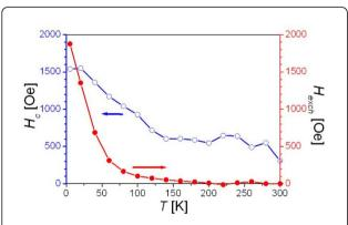
Figure 7 Magnetic hysteresis loops for the samples with 75% of FeO. Coercivity  $H_c$  and exchange bias  $H_{\rm exch}$  of Fe<sub>3</sub>O<sub>4</sub>/FeO composite particles as a function of temperature.
