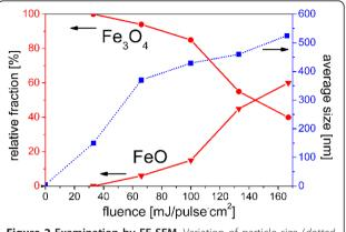
**Figure 2 Examination by FE-SEM**. Variation of particle size (*dotted curve*) and relative fraction of Fe<sub>3</sub>O<sub>4</sub> and FeO with fluence (*solid line*)
