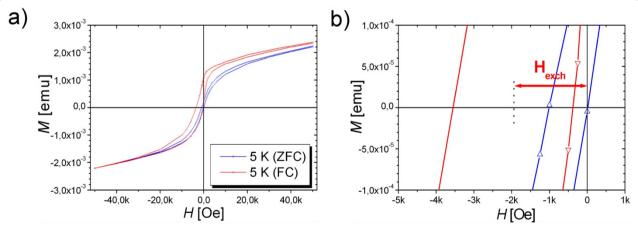
Figure 5 Illustration of the FC and ZFC hysteresis loops. (a) Hysteresis loops of the  $Fe_3O_4/FeO$  particles fabricated at 177 mJ/pulse cm<sup>2</sup>. FC means that the sample is cooled from 300 to 5 K in the 50 kOe field. (b) The magnification around origin of hysteresis loops of the  $Fe_3O_4/FeO$  particles fabricated at 177 mJ/pulse cm<sup>2</sup>.
