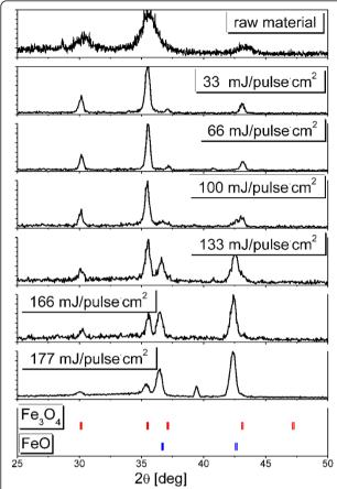
**Figure 3 X-ray diffraction patterns of raw magnetite and irradiated nanoparticles at various laser fluencies.** Standard XRD peaks for Fe<sub>3</sub>O<sub>4</sub> and FeO are plotted for reference.
