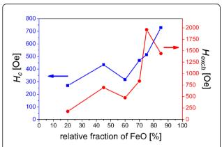
**Figure 6 Variation of H\_c and H\_{\rm exch}.** Coercivity  $H_c$  and exchange bias  $H_{\rm exch}$  of Fe<sub>3</sub>O<sub>4</sub>/FeO composite particles as a function of relative fraction of FeO in particles measured at 5 K.
