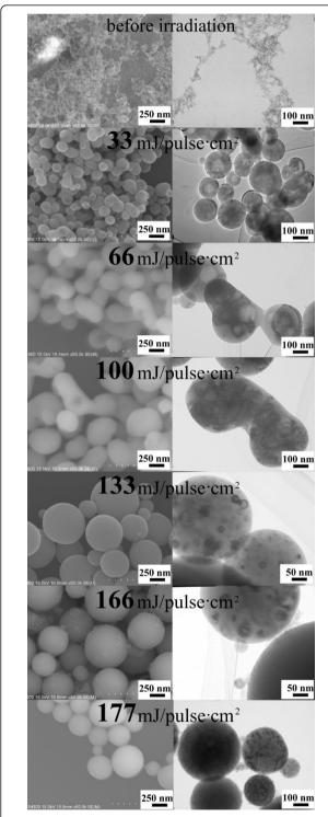
**Figure 1 FE-SEM and TEM images of iron oxide nanoparticles.** Before and after laser irradiation with various fluences.
