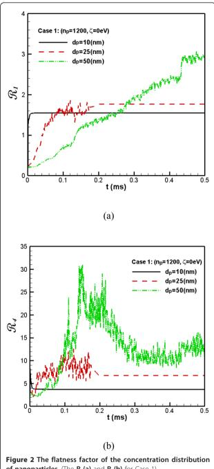
of nanoparticles. (The  $R_1(a)$  and  $R_4(b)$  for Case 1).
