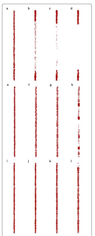
**Figure 1 Snapshots of simulation results.** (Case 1 for d = 10 nm **(a-d)**, d = 25 nm **(e-h)**, d = 50 nm **(i-l)** at t = 0, 5, 10, and 50  $\mu$ s respectively).
