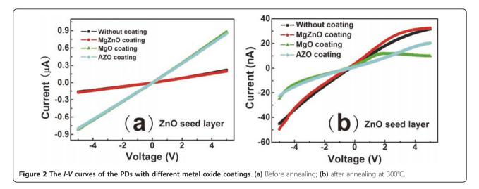
can be collected by Pt electrode at forward bias. However, for PDs without oxide coatings, the contacts at Pt/ ZnO NRs interfaces are improved by annealing process, and the photogenerated electrons can easily reach to Pt electrode at forward bias and get high photocurrent, and PDs without oxide coatings show fast response and recovery behavior after annealing. Therefore, it is concluded that the PDs without oxide coatings display better performance than those with oxide coatings.
