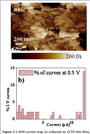
I-Vs acquired in a  $10 \times 10$  matrix and its distribution histogram
