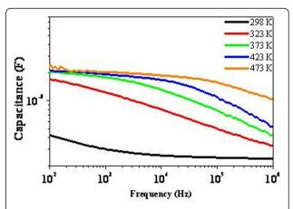
Figure 2 C-f curves at different temperatures on the asfabricated Pt/CCTO/IrO<sub>2</sub> capacitors.
