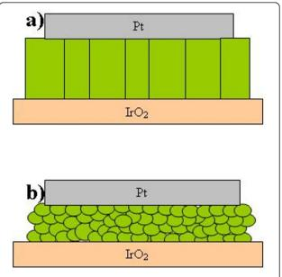
Figure 1 Schematic cross section of CCTO thin films possessing columnar (a) and "bricks wall" like (b) morphologies.
