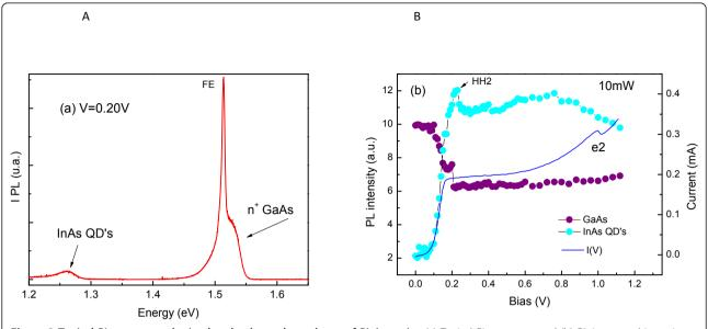
Figure 3 Typical PL spectrum obtained and voltage dependence of PL intensity. (a) Typical PL spectrum and (b) PL integrated intensity as a function of applied voltage at 2 K, for B=0 T and 10-mW laser excitation.
