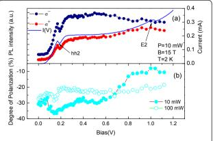
Figure 5 Polarization of the injected carriers. (a) Integrated PL intensity of QD emission as a function of applied voltage at 15 T. (b) Circular polarization degree of QD emission for lower and higher laser intensity as function of applied voltage at 15 T and 2 K.
