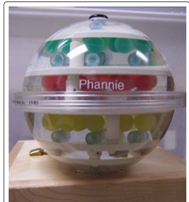
Figure 1 NIST/ISMRM system phantom to measure T1, T2, proton density and geometric distortions.
