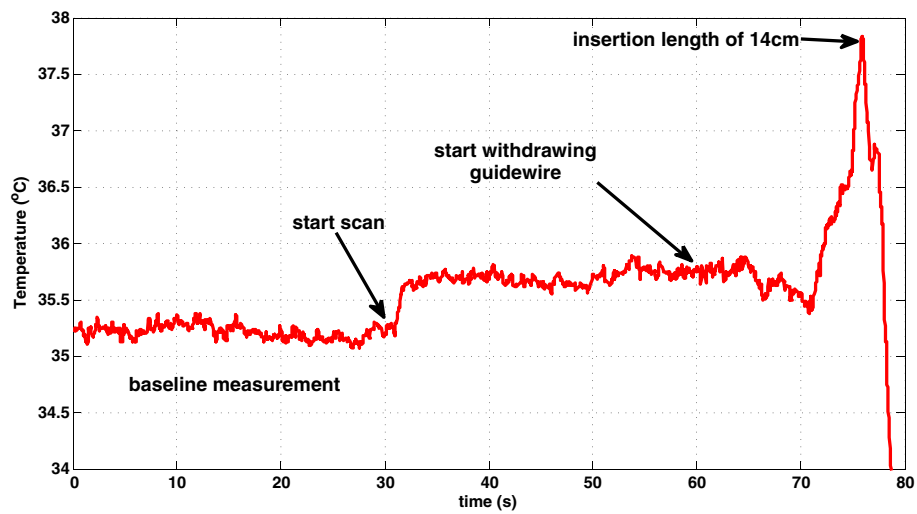
Figure 6 A representative in vivo temperature recording during manual pullback. The flip angle is increased to 90°; SAR, 3.96 W/kg to exaggerate heating. A temperature baseline is obtained before scanning begins. Scanning generates a small temperature rise. After a further interval, the guidewire is withdrawn from the aortic arch during bSSFP MRI. Noteworthy heating was observed just as the guidewire tip entered the tip of the vascular introducer sheath at an insertion length of 14 cm.
