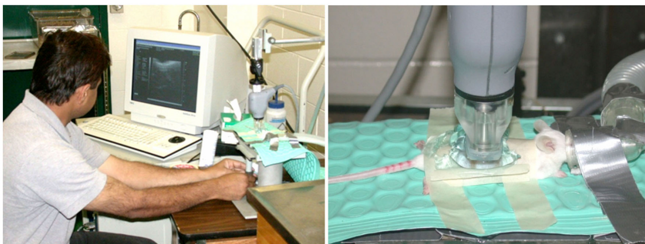
Figure 1 Ultrasound imaging of the ovaries of anesthetized mice by transcutaneous ultrasound bio-microscopy using a 40 MHz transducer.
