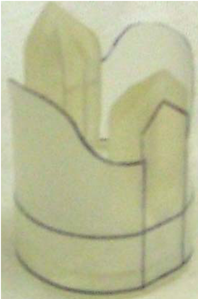
Figure 4 Actual 2:1 scale device with optimized frame and shaped Biospan® leaflet. A threaded extension from the base (not shown) screwed into the test section fixture to improve alignment and prevent leakage.
