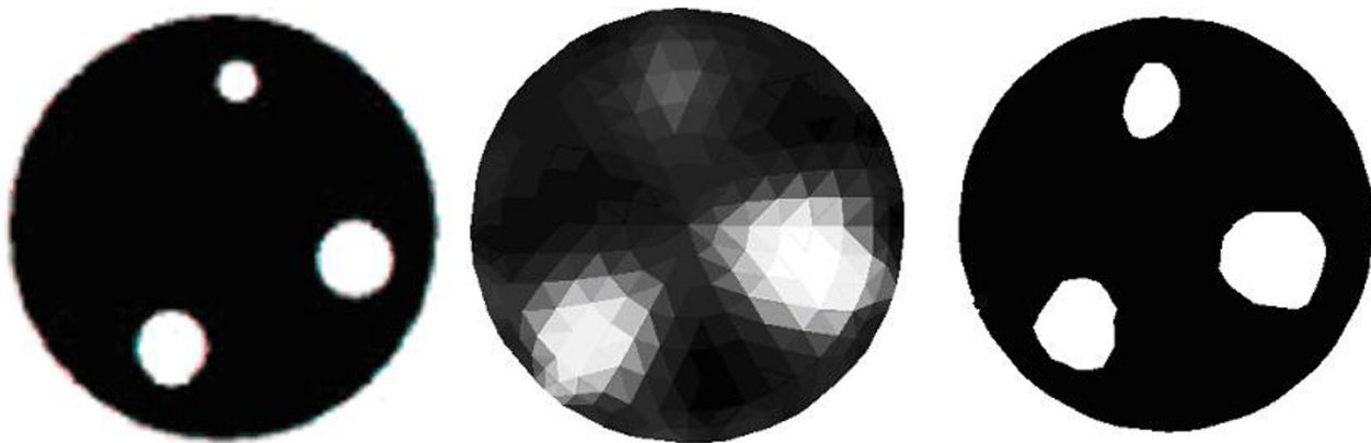
Figure 4 A 2D example with the truth with three inclusions (left), a standard reconstruction (centre) and a level-set reconstruction (right).
