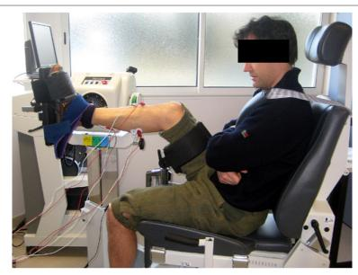
**Figure 4 Appearance of the experiment.** The torque around the ankle joint was measured along with EMG of medial gastrocnemius (GAS) and soleus (SOL) during voluntary plantar flexion.
