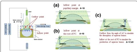
**Figure 2 Connection diagram of experimental apparatus. (a)** inflow point along the pupillary margin; **(b)** inflow point at the root of PC; **(c)** intraocular flow measurement in symmetry AC.
