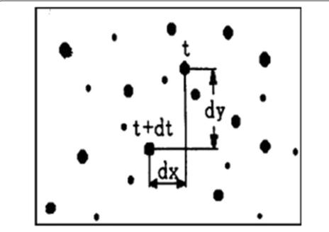
Figure 1 Principle of PIV velocity measurement.
