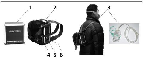
**Figure 2 Production of oxygen enrichment device.** 1) machine body; 2) bag; 3) disposable medical oxygen mask; 4) battery; 5) switch; 6) joint of oxygen enriched air outlet.
