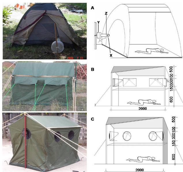
Figure 1 Furvela trap (A), Ifakara A tent trap (B), Ifakara B tent trap (C), with section drawing of each. The human occupant is protected from mosquito bites by a netting panel within the Ifakara A and B designs. For the Furvela trap, mosquitoes approach the small opening in the tent zipper (X) where they are drawn into the collection bag collection bag (Y) when they pass the CDC light trap entrance (Z), while in the Ifakara designs they enter through a funnel shaped entrances tilted upward. All dimensions in mm.
