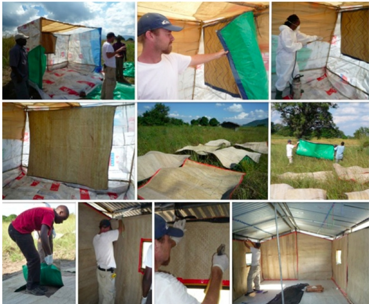
Figure 1 Spraying palm woven mats with DDT. Palm woven mats previously cut out to fit on the walls of experimental huts were sprayed with 2 g/m 2 DDT. Spraying was conducted in a temporary structure that was later burnt. Spraying the mats instead of the walls ensured that mats could be moved easily from one hut to another without contaminating the walls. This allowed rotation of treatments between huts.
