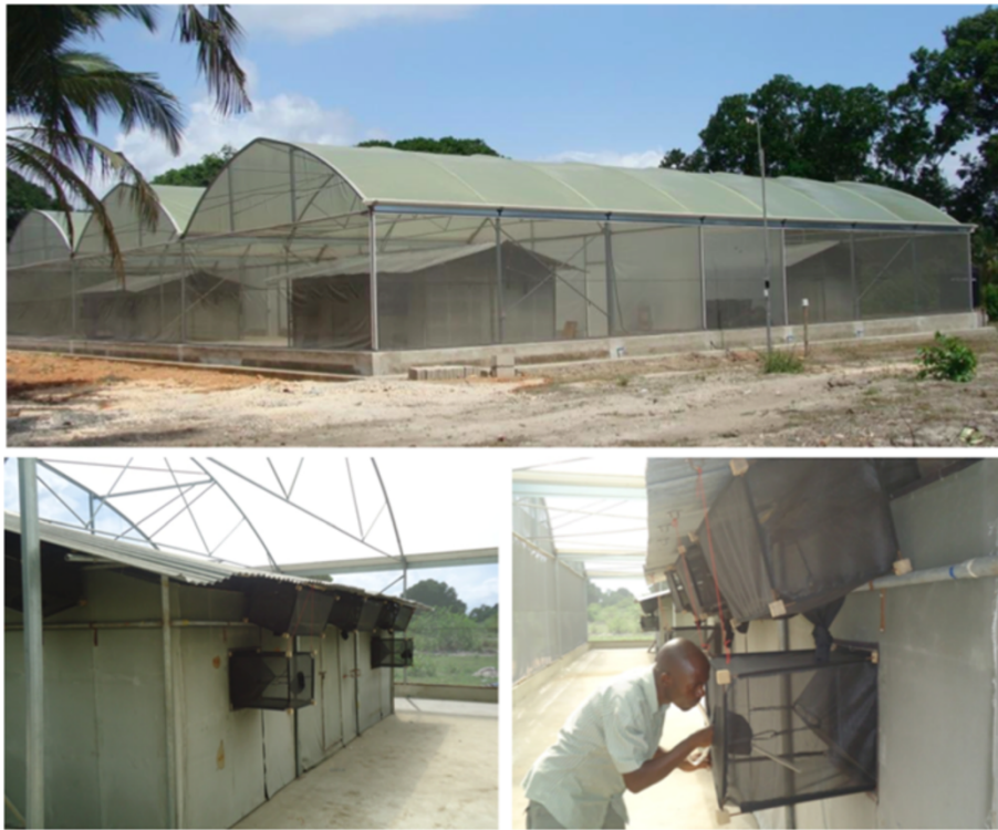
Figure 4 Semi-field system. The walls and the roof of the semi-field system (SFS) are made of metal frames and fibreglass netting material. It was divided into four equal square sections divided by fibreglass netting. An experimental hut was placed in each compartment. The SFS [14] allowed replication of experiments within a short period of time. Laboratory reared mosquitoes were used and were available throughout the duration of experiments hence there were no delays as usually experienced in the field.
