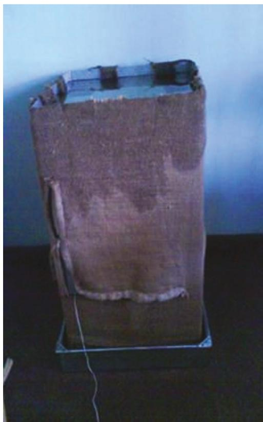
**Figure 1** Evaporative cooler box with drip tray.
