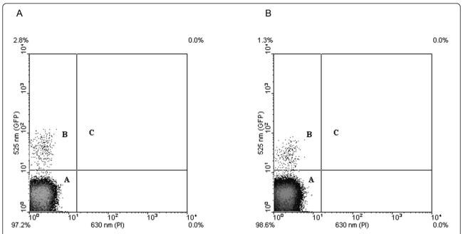
**Figure 2 Antifoams do not affect cell viability.** Viable cells without antifoam (A) and with 0.6% Antifoam A (as a representative example; B) are shown. Population A, which is not cellular, comprises events that are related to electronic and particulate noise. Population B comprises cells with enhanced green fluorescence due to the expression of GFP. Population C is where any dead cells (stained red with propidium iodide) would be observed.
