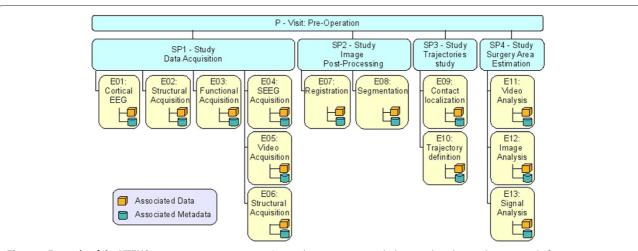
Figure 1 Example of the XTENS process-events structure. A complex process can include several studies, each composed of atomic events.
