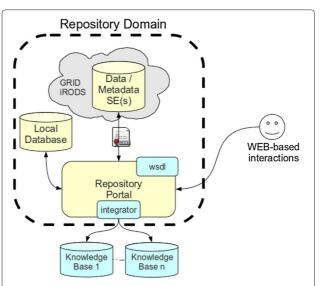
**Figure 2 XTENS overall architecture.** The repository is accessed through a web portal interacting both with a local database for patient metadata and with a Grid based Storage Element.
