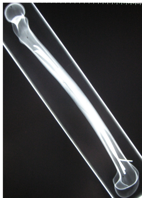
Figure 2 Radiograph (lateral view) of a 3CL femoral model with retrograde intramedullary nailing, showing two 3.5 mm titanium nails implanted in 2C shaped configuration and one additional 2.5 mm titanium nail implanted antero-lateral.
