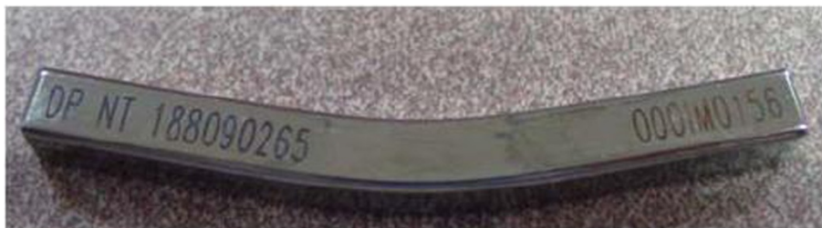
Figure 1 Square, anatomically shaped NiTi alloy spinal rod.
