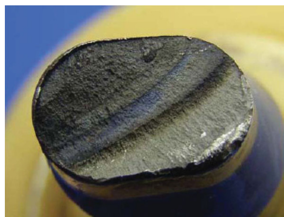
Figure 8 Fatigue fracture surface of a clinically failed titanium neck adapter.
