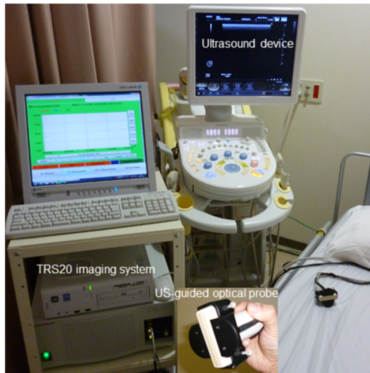
Figure 1 A dual-channel TRS system. The patient lies in the supine position on the bed. A US-guided optical probe from the TRS imaging system (TRS20, Hamamatsu Photonics K.K., Japan) is used to acquire measurements of a patient's breast and define an ROI in which the breast lesion can be measured.
