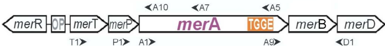
Figure 4 Schematic representation of a typical broad-spectrum mercury resistance operon of Gram-negative bacteria and the location of primers (arrowheads) used for amplification of merA . The merA stretch used for TGGE analysis is marked orange. R, regulator protein merR ; OP, operator/promotor region and start of transcription; T, periplasmic transport protein merT ; P, membrane bound transport protein merP ; A, mercuric reductase merA ; B, mercuric lyase merB ; D, regulatory protein merD .
