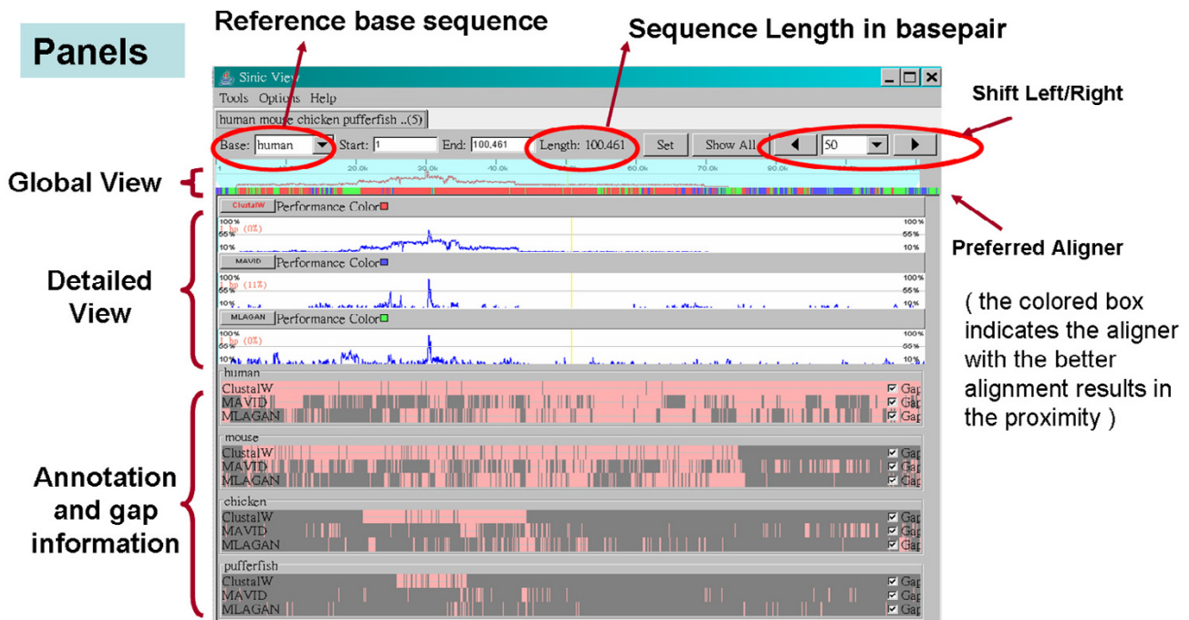
Figure 1 The screenshot shows the user interface of SinicView. The alignment result is of the SCL gene regions in human, mouse, chicken, pufferfish, and zebrafish. Three alignment results of five sequences aligned by ClustalW, MAVID, and MLAGAN are shown.
