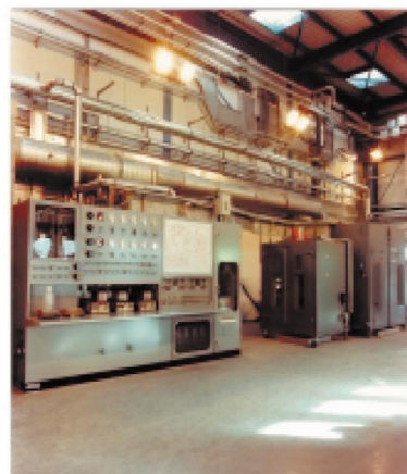
Fig. 2 Diagram of the core-flood experimental set-up, with the actual lab set-up shown right. The core-flood cell was maintained at 7000 psi confining pressure and 70 °C. Pressure differential across P_0/P_1 = 700 psi.
