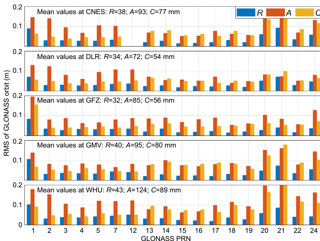
Fig. 6 RMSs of GLONASS orbit products in along-track, cross-track, and radial directions from different ACs (mean RMS of orbit errors for all GLONASS satellites is shown in each subplot)
