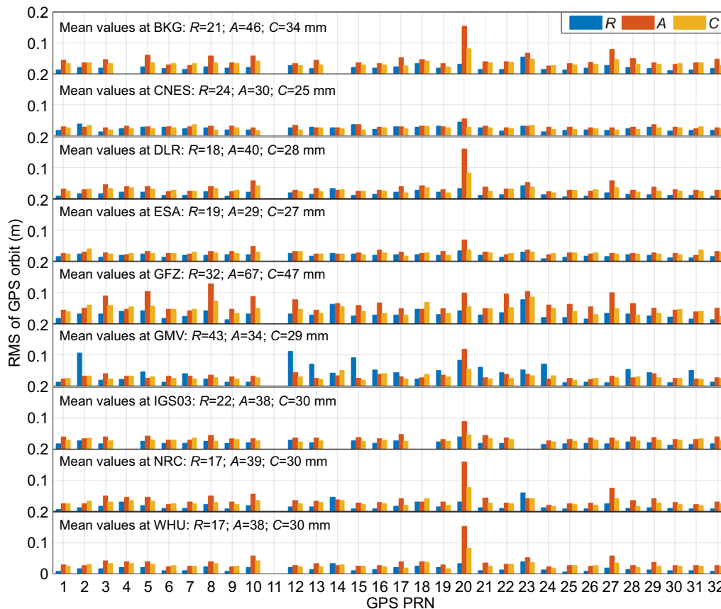
Fig. 2 The RMS values in the radial (R), along-track (A), and cross-tracks (C) directions of GPS real-time orbit from different IGS ACs (mean RMS of orbit errors for all GPS satellites is shown in each subplot)
