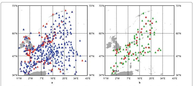
Fig. 2 The EPN [blue] and SONEL [red] networks in Europe provide PPP-RTK service in (a). In this study, they are mainly used to generate the ionosphere precision map and regional troposphere model. The red stars denote for assessing the PPP-RTK performance and the green triangles denote for the nearby reference stations in (b) which provide the interpolated ionosphere for the user stations
