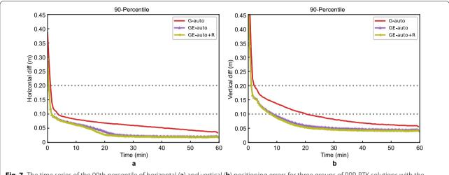
Fig. 7 The time series of the 90th percentile of horizontal (a) and vertical (b) positioning errors for three groups of PPP-RTK solutions with the proposed dynamic ionosphere stochastic model
