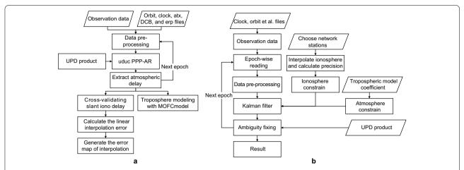
**Fig. 1** Flowcharts of the network and the user platforms of the PPP-RTK software and algorithm. The subgraph **a** is the processing strategies on the server side, and the subgraph **b** is the processing strategies on the user side
