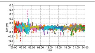
**Fig. 5** The slant single-differenced-between-satellite ionospheric delay interpolation error for user site MALA in Spain, 03 August 2021 (DOY 215). Different colors represent different satellites
