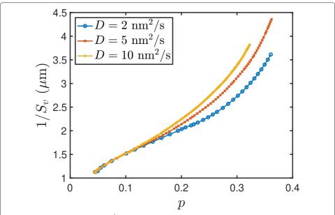
**Fig. 5** Characteristic length scale  $S_v^{-1}$  for varying simulated diffusivities (initial conditions of configuration 1).  $S_v^{-1}$  remains an order of magnitude smaller than the simulation domain size  $L_x = 72 \ \mu \text{m}$
