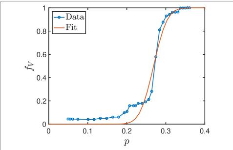
**Fig. 8** Fraction of total bubble volume that is connected to a free surface,  $f_V$ , as a function of porosity p for M = 1, Configuration 1, and function fit to the data using Eq. (13)
