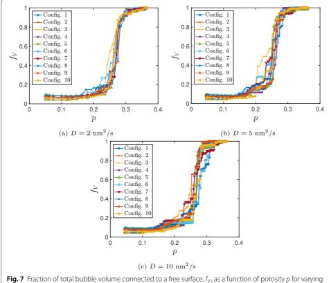
**Fig. 7** Fraction of total bubble volume connected to a free surface,  $f_V$ , as a function of porosity p for varying diffusivity
