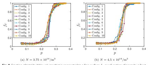
**Fig. 9** Fraction of total bubble volume that is connected to a free surface,  $f_V$ , as a function of porosity p for **a**  $N = 3.75 \times 10^{14} / \text{m}^3$  and **b**  $N = 4.5 \times 10^{14} / \text{m}^3$ , with  $D = 2 \text{ nm}^2 / \text{s}$
