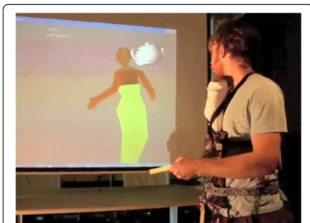
**Fig. 5** In the teapot touching intervention, the camera flies around the virtual avatar, continuously altering the spatial relationship between the avatar and player. The player must perform mental rotation to use the puppet controller to make the avatar touch teapots as they appear
