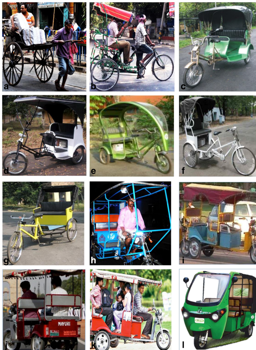
Fig. 5 The evolution of pulled rickshaws through various innovations. a Conventional hand-pulled rickshaw (Ganguly 2014). b Conventional cycle rickshaw (source: author's own). c-g Soleckshaw prototypes Mark-1 Series-1, Mark-1 Series-2, Mark-2 Series-1, Mark-2 Series-2 and prototype with motor below the seat, respectively (source: CSIR-CMERI). h Low-cost Mark-2 lookalike rickshaw on the roads of Kolkata, India (source: author's own). i-k Modified models of various electric rickshaws on the roads of Delhi (Sengupta 2013; Angre 2014; MT 2014). l Kinetic Safar (source: Kinetic Green)
