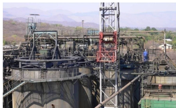
Fig. 1 Commercial-scale BIOX ® bioleaching process in Barberton, South Africa (Kaksonen et al. 2014). [Image courtesy of Dr. Anna H Kaksonen, The Commonwealth Scientific and Industrial Research Organization, Australia]
