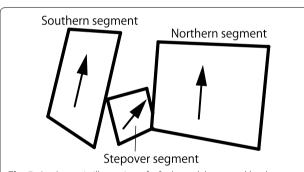
**Fig. 5** A schematic illustration of a fault model ruptured by the 2018 Hokkaido Eastern Iburi earthquake. The view point is located northeast of the focal area. Arrows indicate the motion of the hanging wall of individual faults
