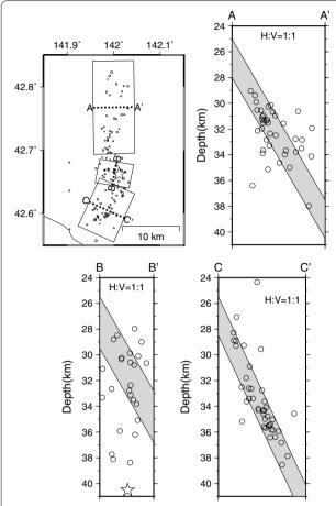
**Fig. 3** Vertical cross sections in the northern segment (A–A'), in the stepover segment (B–B'), and in the southern segment (C–C'). All sections have no vertical exaggeration. A total of 118 aftershocks were selected from the hypocenters in Fig. 2a from 2018-09-06 03:15 to 2018-09-06 09:00. Shaded areas indicate zones with dip angles of 60°, 60°, and 65° in the A–A', B–B', and C–C' sections, respectively
