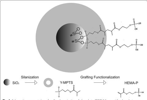
**Fig. 1** Schematic representation of graft polymerization of phosphate (POOH) from acidic phosphate monomer (HEMA-P) on  $SiO_2$  nanoparticles. The grafting of POOH on the  $SiO_2$  nanoparticles was carried through a silane-coupling agent (y-MPTS)
