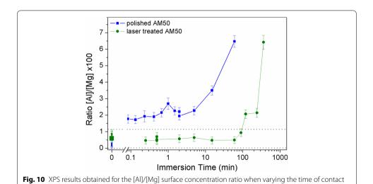
between a polished AM50 surface or a laser-treated surface and a water film
