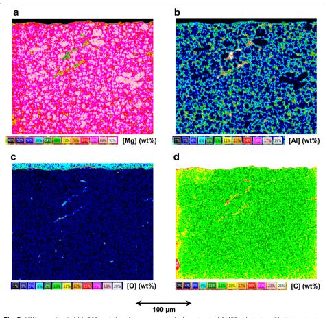
**Fig. 3** EDX mapping (width 260  $\mu$ m) showing a crosscut of a laser-treated AM50 substrate, with the treated surface oriented towards the *top*, in contact with an embedding compound containing filler particles. *Maps* indicating the distribution of **a** magnesium, **b** aluminum, **c** oxygen, and **d** carbon based on the respective  $K_a$  X-ray series are displayed, and the concentrations [Mg], [Al], [O], and [C] are given in weight% (wt%)
