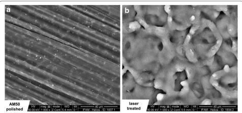
**Fig. 8** SEM images obtained with a primary electron energy of 30 keV and also collecting back-scattered electrons from **a** a polished AM50 substrate surface and **b** a laser-treated AM50 surface
