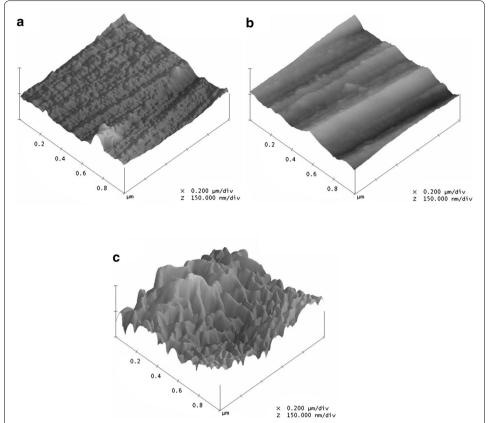
**Fig. 5** SFM images of grain surfaces imaged on **a** a polished AM50 surface, **b** an AM50 surface immersed in aqueous laccase formulation for 15 s and **c** an AM50 surface immersed in water for 15 s
