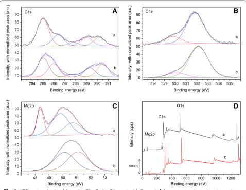
**Fig. 9** XPS results obtained for **a** the C1 s, **b** the O1 s, **c** the Mg2p, and **d** the survey regions when investigating a polished AM50 surface (**a**) or a laser-treated surface (**b**). The intensities for the detail plots **a**, **b**, and **c** are normalized with reference to the respective total signal area
