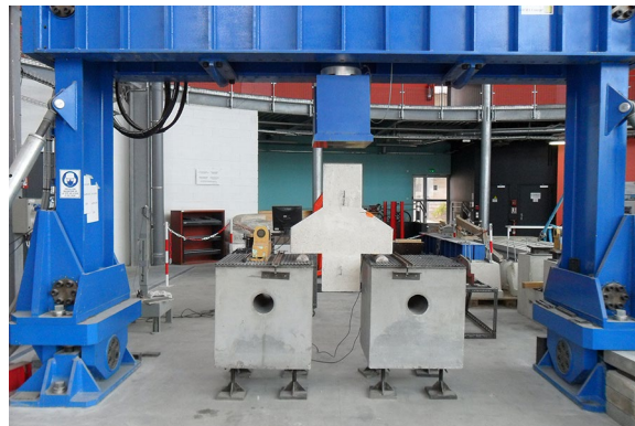
Fig. 2 Flexure bending test of strengthening reinforced concrete corbel
