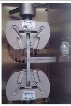
**Fig. 3** DCB specimen and environmental chamber
