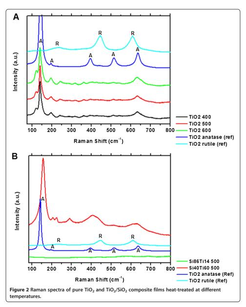
effect under UV light. The photocalytic effect was more pronounced on the sample that had higher Ti content. The  $\rm Si_{86}Ti_{14}$  composite exhibited good hydrophilicity and also photocatalylic effect according to our preliminar photocatalitic tests although the anatase phase was not present. Further studies will be conducted to understand better this phenomenon.
