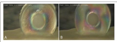
**Figure 1 Photoelastic images.** Representative images of the Filtek Z-350 **(A)** and Filtek Silorane **(B)** specimens captured by the polariscope software after stress analysis. The software registered the value of stress in MPa on the figures.
