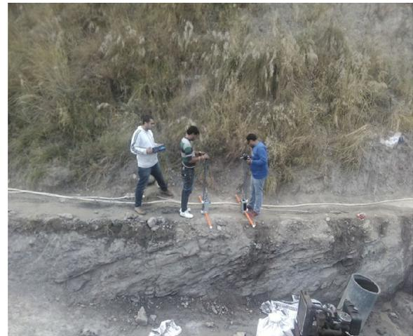
**Fig. 2** A typical set of GPR testing conducted at Mansadevi landslide
