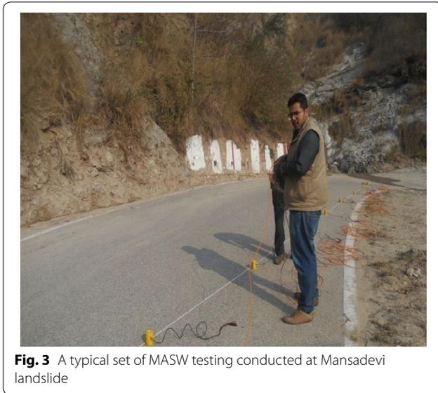
**Fig. 3** A typical set of MASW testing conducted at Mansadevi landslide
