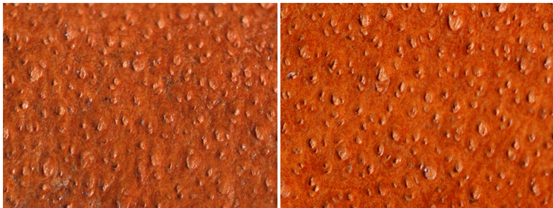
Fig. 6 (Left) An effective non-complete laser cleaning result for removal of soiling particles on the historical vegetable tanned leather surface using ps emitting at 1064 nm using fluence 2 \text{ J cm}^{-2} and 1 scan (OM 10x). Right satisfactory cleaning results for removal of soiling particles on the historical vegetable tanned leather surface using ps emitting at 1064 nm using fluence 2 \text{ J cm}^{-2} and 3 scans OM 10x)
