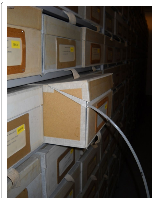
Fig. 2 Field studie on measuring the mercury concentration inside a herbarium box. Example of direct sampling of air
