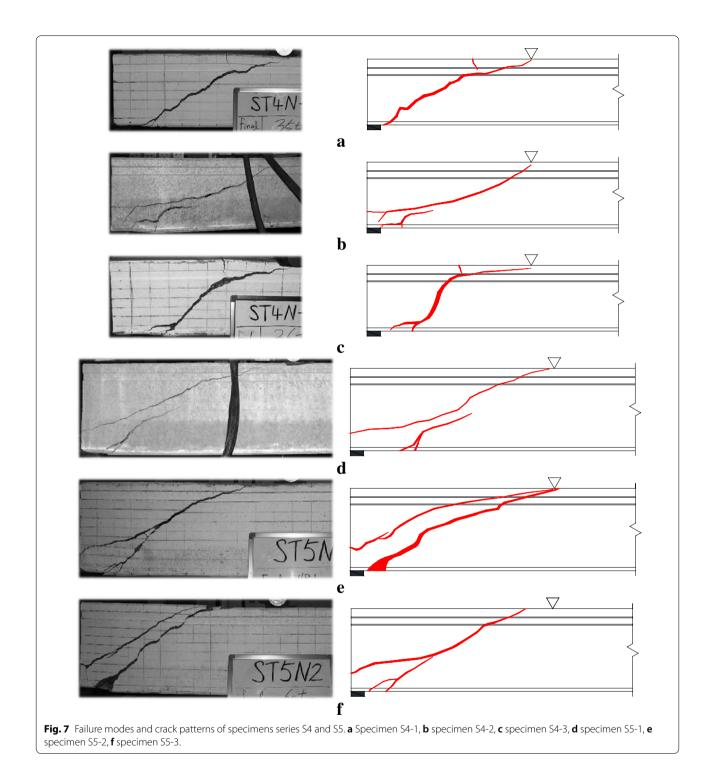
were very similar to the S4 series specimens. The S5 series specimens also showed brittle web-shear failures at 427.2, 454.4, and 369.8 kN, respectively. The average shear capacity was 417.1 kN, which is almost identical to that estimated by the ACI318-05 shear equation.
