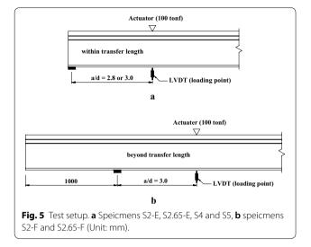
span-depth ratio (a/d) of the S2 and S2.65 series was 3.0, and the one point load was applied on the top of the specimens. The S4 and S5 series were also tested within the transfer length with a shear-span ratio (a/d) of 2.8 as done in the S2-E and S2.65-E specimens, as shown in Fig. 5a.
