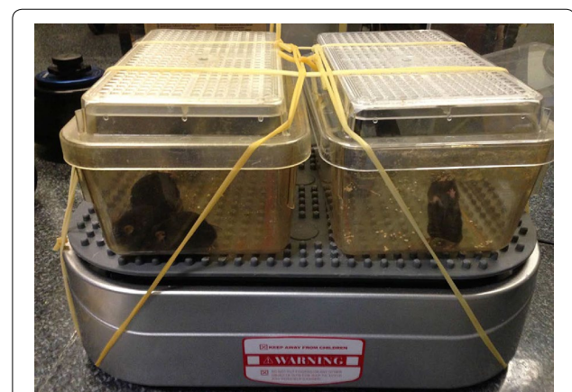
Fig. 1 Picture of vibrating platform capable of delivering the prescribed high frequency, low amplitude vibration ("Methods")
