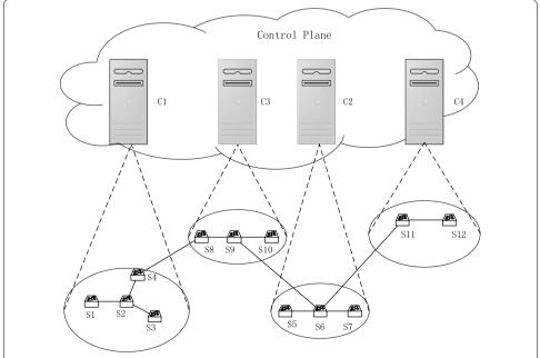
**Fig. 1** The result of DPC algorithm acting on network topology. It is a diagram which is about the relationship between the SDN and optimized DPC algorithms
