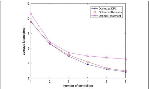
**Fig. 6** Average latency of three algorithms with different controller numbers. *x* axis: number of controllers. *y* axis: average latency (ms): The figure shows that the average communication delay on the OS3E topology is calculated by the optimized DPC algorithm, the optimized k-means algorithm and the optimal placement algorithm respectively. And then, the data values we calculated by these algorithms are compared with each others
