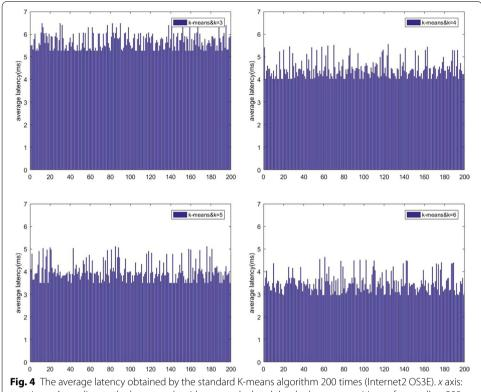
**Fig. 4** The average latency obtained by the standard K-means algorithm 200 times (Internet2 OS3E). *x* axis: test times: According to the k-means algorithm, we calculated the deployment positions of controllers 200 times when the number of controllers is 3, 4, 5 and 6. *y* axis: average latency (ms)
