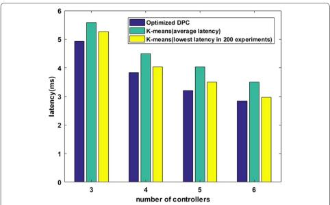
**Fig. 5** Comparison of latency under different algorithms. *x* axis: number of controllers. *y* axis: latency(ms): Among the 200 experimental data obtained by K-means algorithm, we calculate the average communication delay and the minimum communication delay, and compare these data with the optimized DPC algorithm
