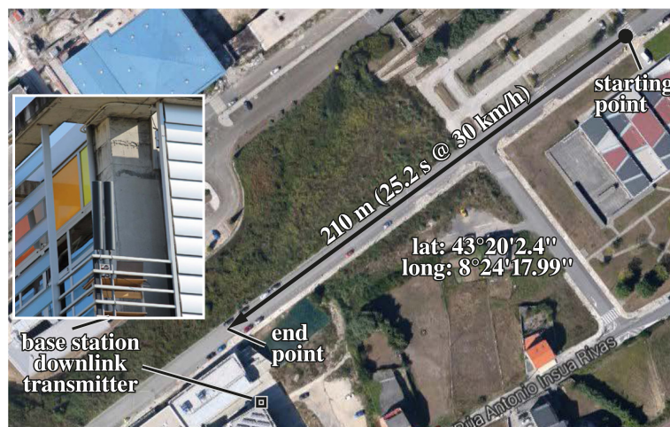
Figure 5 Measurement scenario at the Campus de Elviña, A Coruña. The measurement trajectory as well as the location of the base station are specified.
