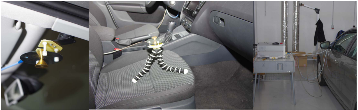
Figure 2 Images of the conical monopole antenna, measurement position, and four-port VNA. [left] Detail of the conical monopole antenna mounted on the front windshield. [middle] One measurement position inside the vehicle. [right] Four-port VNA connected with antennas inside the measured vehicle.
