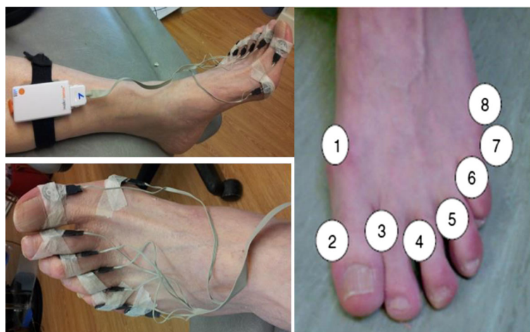
Fig. 2 Walkinsense® sensor placement 1–8 on digital landmarks, as well as experimental set up for data capture. Micropore was loosely applied to secure the sensors
