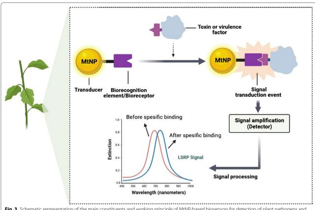
Fig. 3 Schematic representation of the main constituents and working principle of MtNP-based biosensors for detection of plant pathogens and toxins
