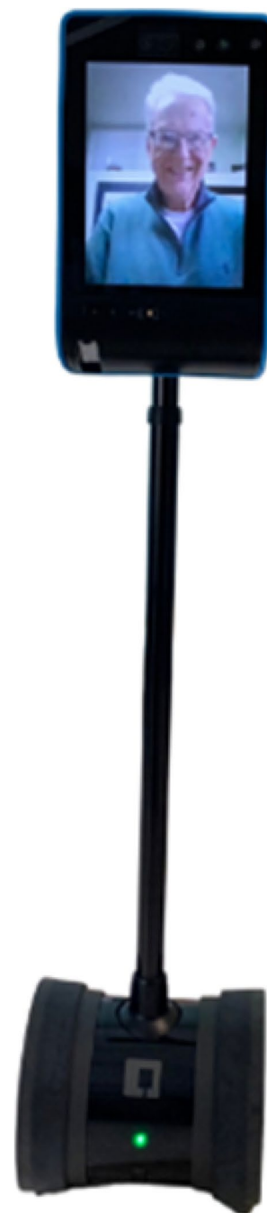
Fig. 1 Atelepresence robot consists of a tablet and wheel attachments
