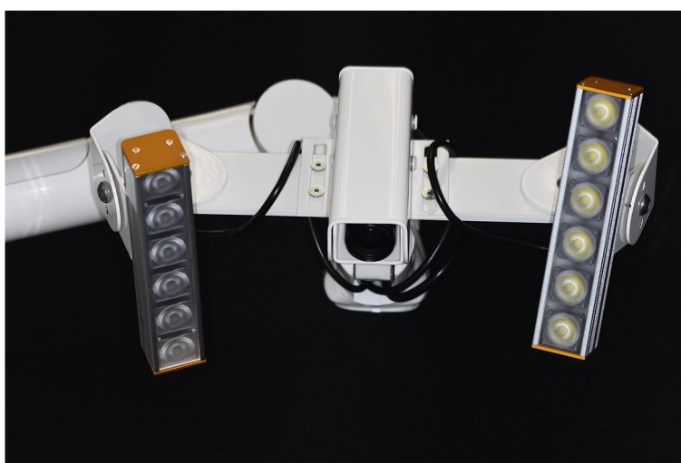
Fig. 4 Bionic Jaw Motion Movement Analyzer. The jaw movement analyzer is composed of a high-speed recording camera and a software running on a computer. The software recognizes the known geometries of the markers and their optical deformation during movement registration thus reconstructing mandibular movement. It is mandatory to check whether the artificial vision software is able to locate reciprocal position of the markers during all opening phases before performing the actual recording (see fail number in Video 1, to ensure the best possible recording no fail should occur)
